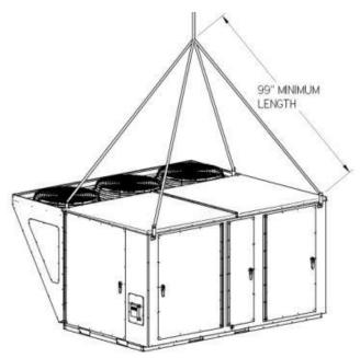
Figure 7 - Lifting Details of a 11-25 and 30 ton Standard or Power Exhaust Unit
