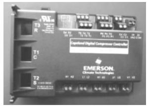
Figure 36 - Variable Capacity Compressor Controller
