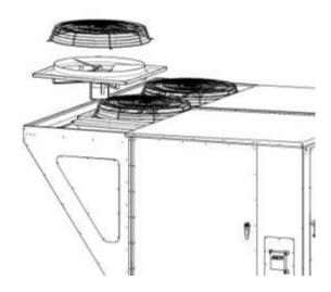
Figure 39 - Removal of a Condenser Fan Assembly
