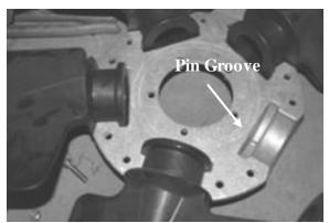
Figure 31 - Pin Groove Location
